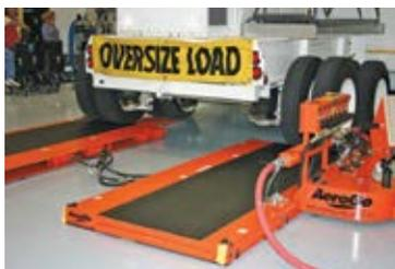
**Eliminate Floor Damage.** Aero-Planks utilize air casters, which distribute the load weight over a larger surface area than with rollers or wheels. Load stress is spread evenly across the surface, eliminating potential floor damage.
