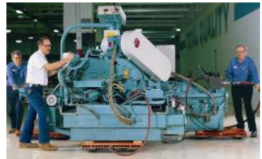
Air Caster Rigging System makes it easy to move machines like the unit shown above.
