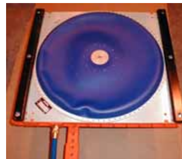
DuraGlide Aero-Caster beneath each end of the Load Beam
