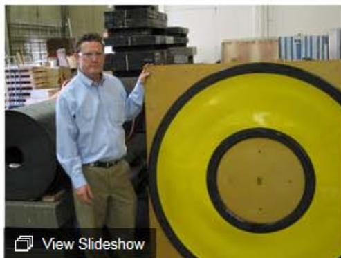
Steve Wilhelm photo One of the inflatable rings that AeroGo fabricates to lift heavy loads, supported by CEO John Massenberg.
