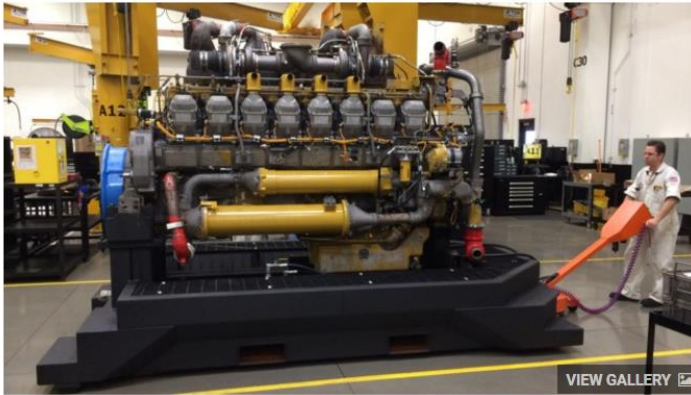
Sole operator moving multi-ton load via air bearing technology.
